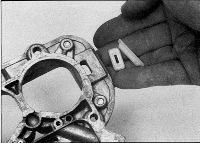
Choke-arm dust seals are held in casting on underside of float bowl. Pry off longer seal: O seal will fall out. Both seals can be re-used.
