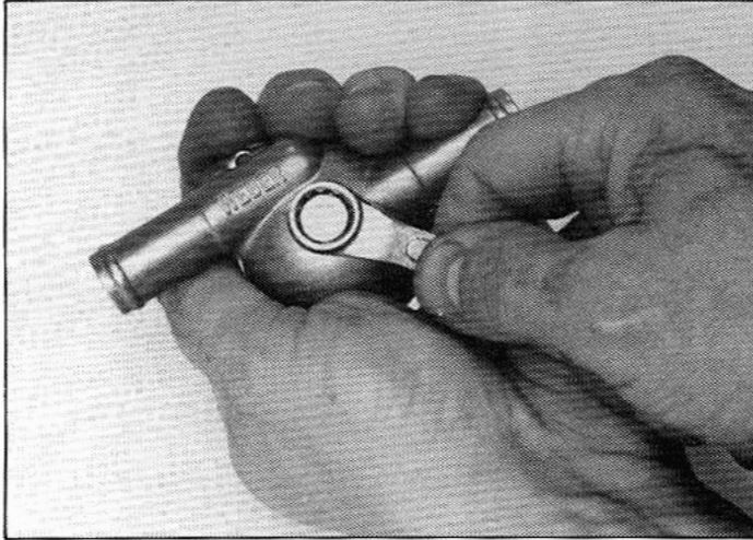
Water chamber comes apart easily by removing 11mm bolt. Unless it leaks, leave chamber assembled.
